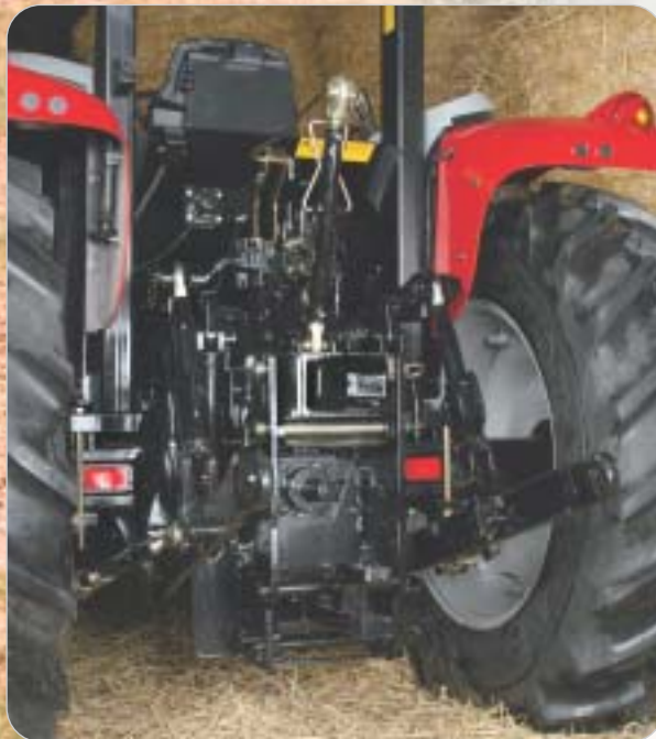
Well specified 3-point linkage and hydraulics for optimum implement compatibility
