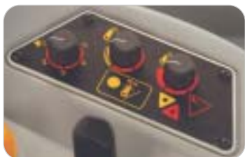
Other ELC functions are set by smooth, rotary controls. LEDs indicate linkage lifting and lowering.
